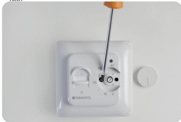
Termoregulators ar noņemtu regulatoru
